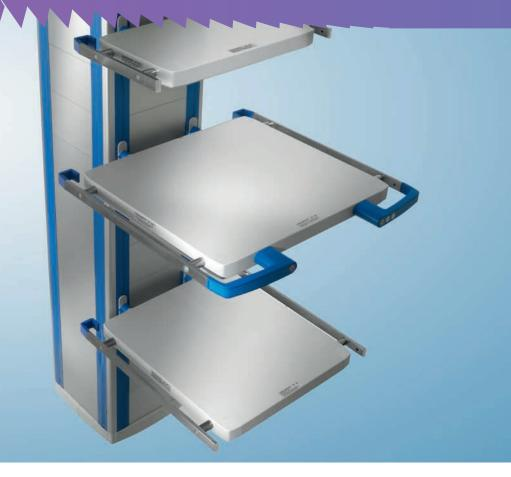
For the TruPort™ Supply Unit we offer shelves in five heavy load versions (HL – 80 kg / 176 lbs) and two medium load versions (ML – 50 kg / 110 lbs) of various sizes. The shelves can be mounted to the system head without tools by means of the click mechanism.
